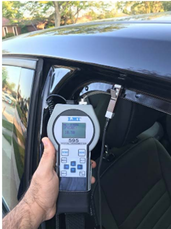
Figure 54. Experimental test for the secondary seal gap
