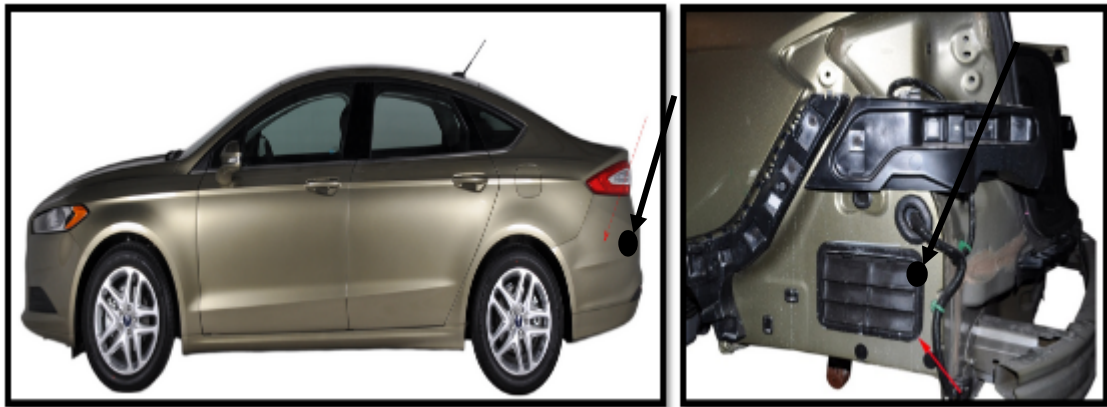
Figure 7. The Air Extractor in the Rear Quarter Panel for a Vehicle
