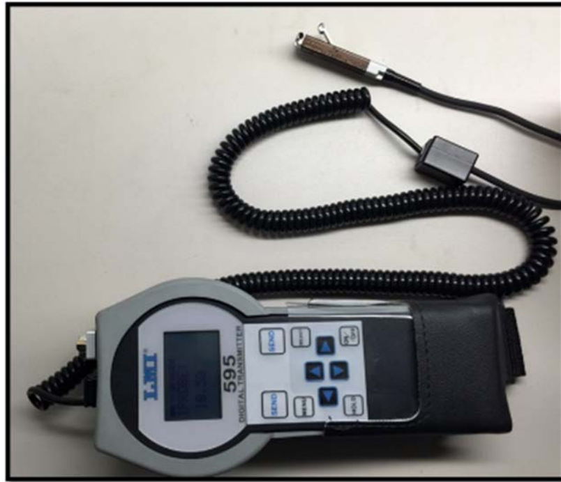
Figure 28. The LMI Device to Measure the Seal Gap for the Secondary Seal
